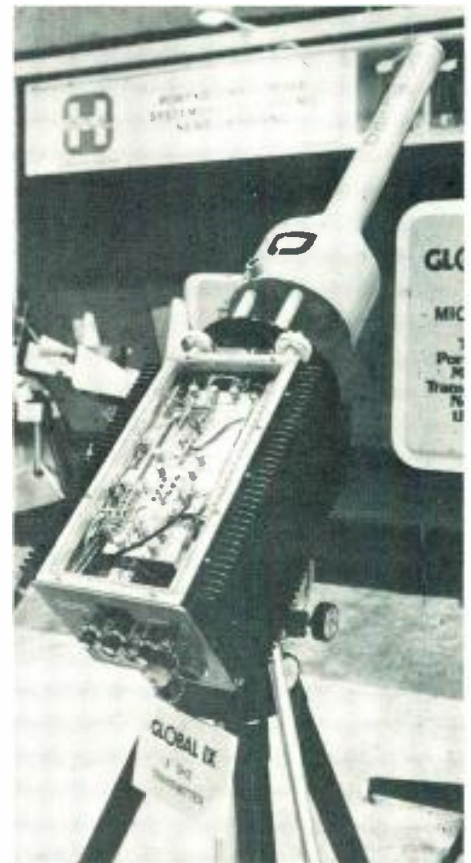
Harris/Nurad Global IX 2 GHz portable.
