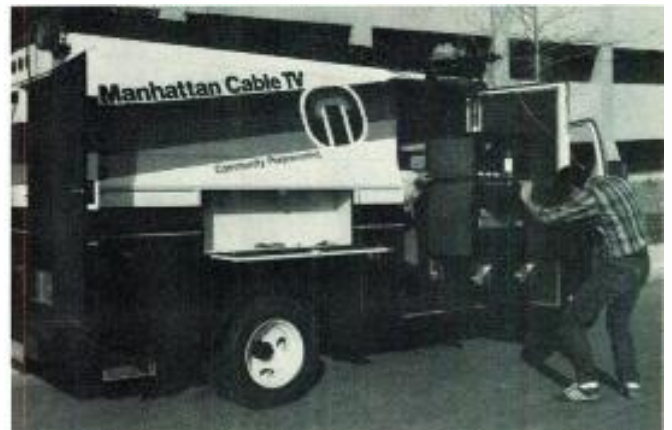
From street to high rise—that's the way Centro designed the van for Manhattan Cable TV's big city needs. Here portable studio equipment is lowered by hoist to go into action in a skyscraper to make good on Manhattan's motto: "The City is our Studio."
