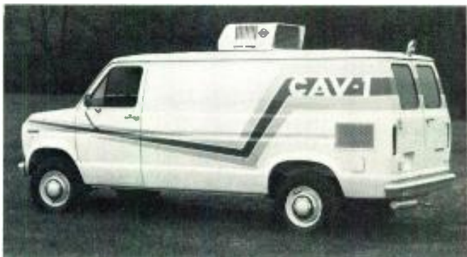
A large number of Cable Access Vans (CAV-1) have been sold by Wolf Coach to operators. This CAV supplied to Continental Cable can carry two to three ENG cameras, plus tape machines, a character generator, and possibly on-board editing equipment.
