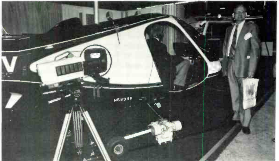
Microwave package for Enstrom bird has Tayburn and BMS components.
